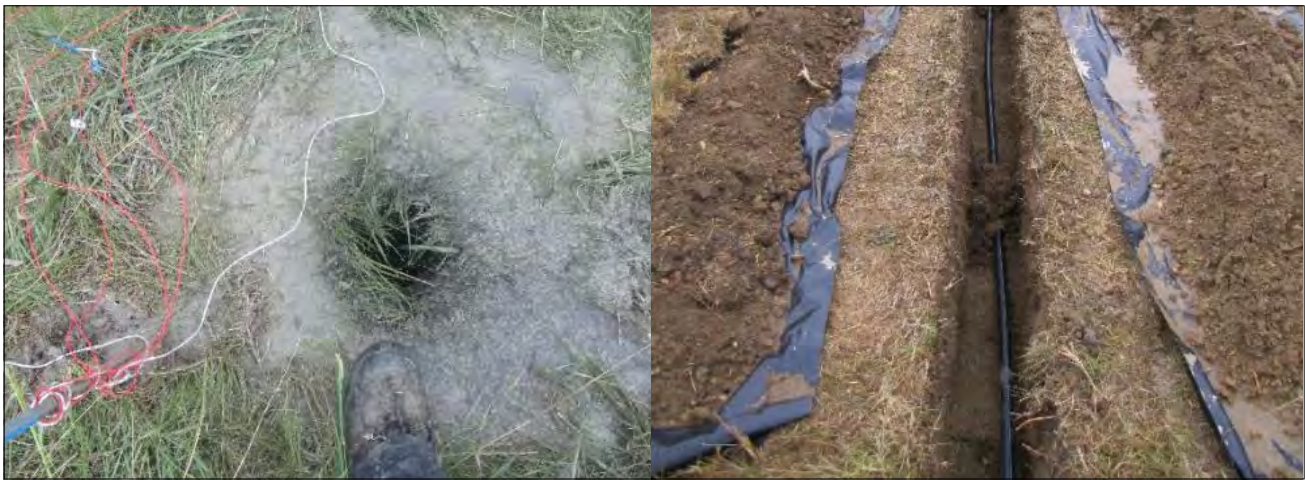
FIGURE 3. Engineered observables generated for testing events. Left: a hole prepared for a chemical explosive to mimic the impact of ground fluffing; Right: Preparatory work to assess the impact of changes to the water table on multispectral signatures.
