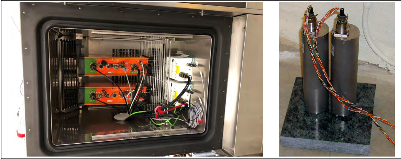
FIGURE 11. Self-noise testing of Q330M+ (Kinematics, USA) and Centaur (Nanometrics, Canada) digitizers inside the temperature chamber at SNL (left panel) and side-by-side testing of two CMG3V vault seismometers at the right panel (courtesy of SNL testing reports).
