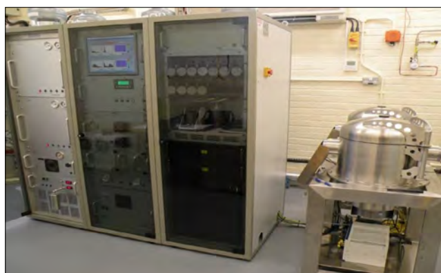
FIGURE 22. The UK CTBT radionuclide noble gas laboratory (GBL15), which uses a SAUNA II IMS lab system to process and measure radioxenon samples from the IMS noble gas station network.
