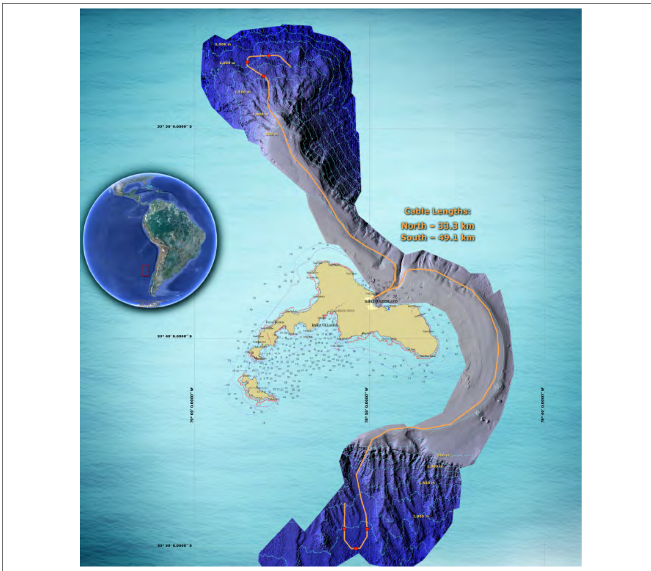
FIGURE 19. HA3 cable routes and triplet locations, as of 2014.
